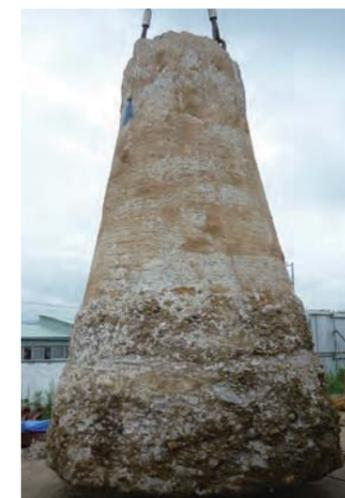
軸部径φ1,300mm/拡底部径φ2,700mm
