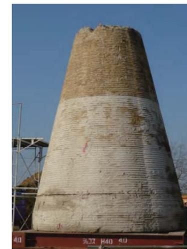
軸部径φ2,000mm/拡底部径φ4,400mm
